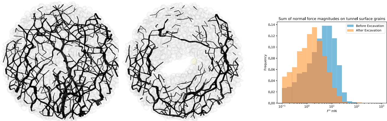
Fig. 5. Change in forces around the tunnel due to ant excavation for the green tunnel in experiment 2 within the bulk. (Left) Intergranular forces in a tunnel cross-section before excavation. (Center) Forces in the same cross-section after tunnel excavation. (Right) Distribution of F_n in particles that make the tunnel surface before and after excavation. The presence of the tunnel has reduced the stress in tunnel particles due to arching, with P \ll 0.005 under the Kolmogorov–Smirnov test.
